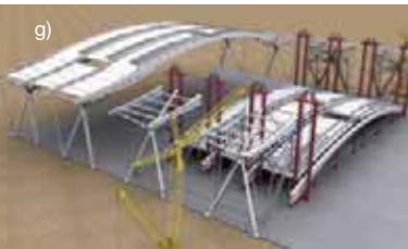
6. Roof assembly sequence.
