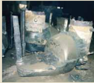
17. Casting removed from sand mould.
